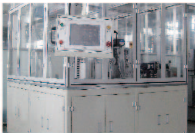
方型锂离子电池极片自动生产线 Prismatic Lithium-ion battery electrode automatic production line
